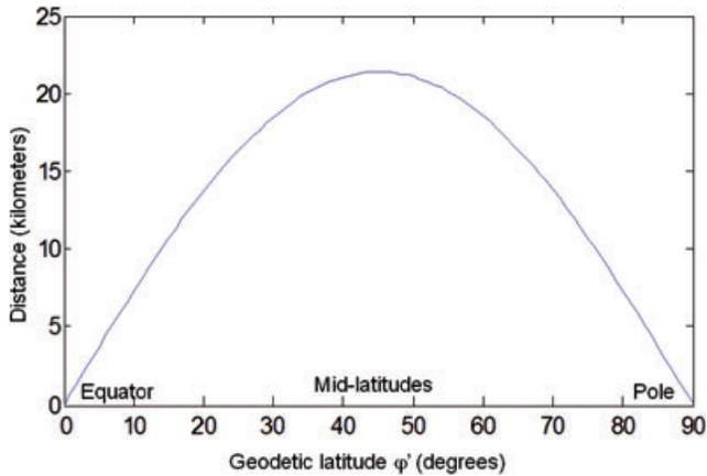
**Figure 5** Distance between points having the same numerical value for latitude depending on whether it is geocentric- or geodetic-based, as a function of geodetic latitude
