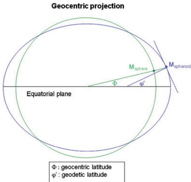
**Figure 6** Geocentric projection of a sphere to a spheroid
