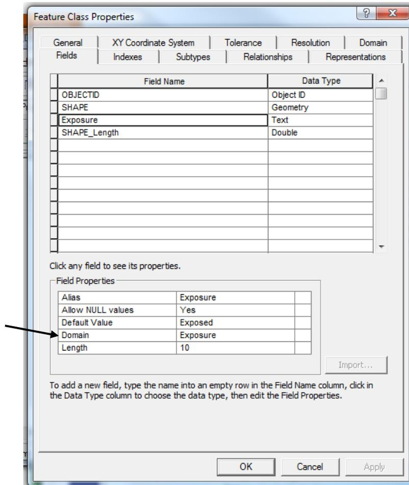
**Figure 12:** Attaching domains to feature classes. The Contact feature class is represented in the figure.
