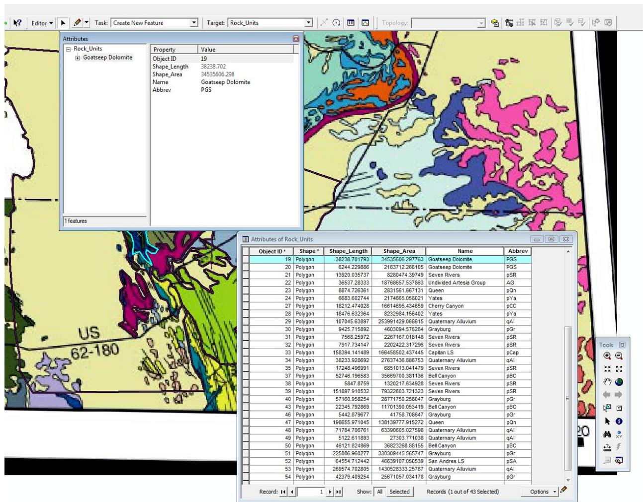
**Figure 18:** Naming the rock unit polygons.
