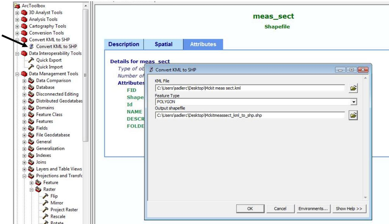
**Figure 7:** Converting the .kml file for my measured sections to a shapefile.
