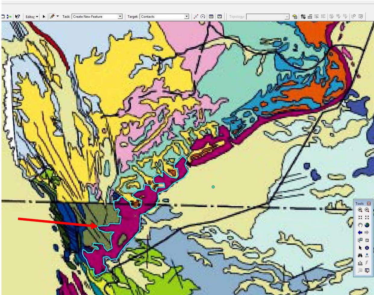
**Figure 13:** Digitizing faults and contacts. Example indicated by arrow is the Capitan LS contact.
