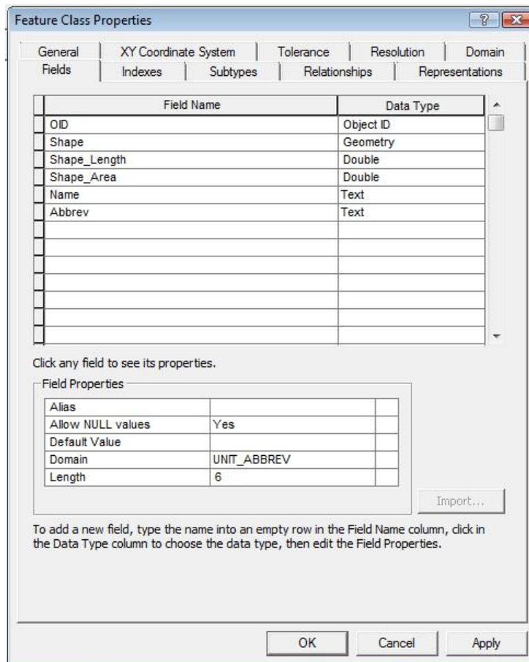
**Figure 17:** Assigning fields and domains to the Rock\_unit feature class.
