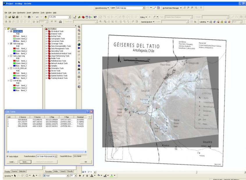
Figure 7: Scanned image being georeferenced to GoogleEarth image
