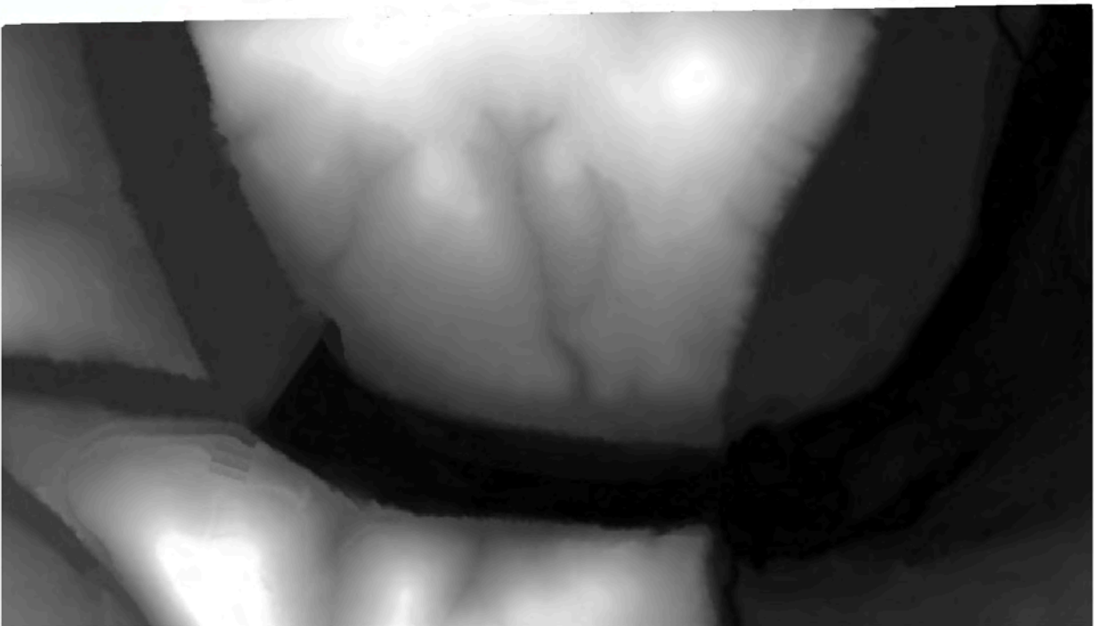
Figure 7. Creating a raster from a TIN and corresponding result I used the TIN to Raster toolbox to complete the conversion. I used the default options for the Output Data Type and Method but changed the Sampling Distance to 4.59 to correspond to the resolution of the LiDAR and I used a Z Factor of 0.3084 to convert the elevation from feet to meters.
