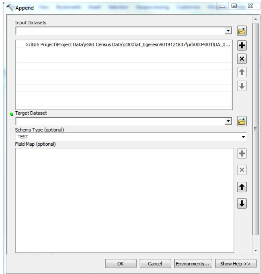
Figure 9. Appending TIGER shapefiles into single layer.
