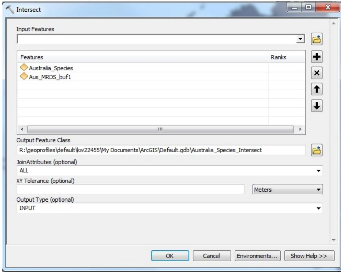
Figure 7. Intersect tool showing the merged Australian species polygon and the buffered Australian mines, with all attributes being joined and the output feature class the same as the input. XY tolerance was disregarded.
