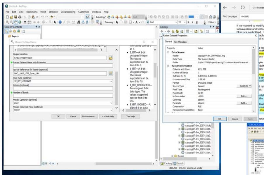
Figure 2. Image showing the Mosaic to New Raster tool in use. The original cell size of the LiDAR data was retained.
