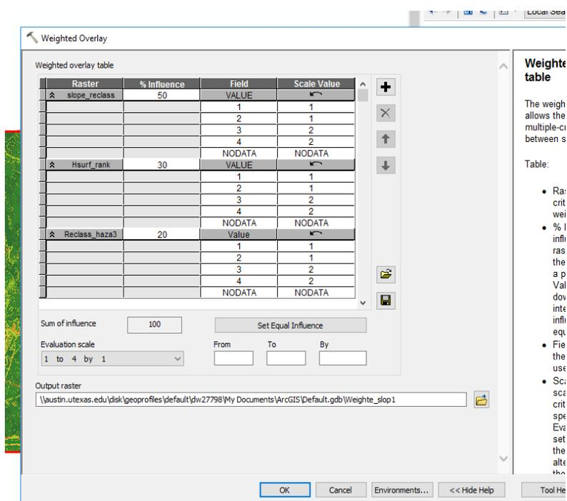
Figure 14. Weighted Overlay Analysis tool re-ranking every input raster for a suitability raster.
