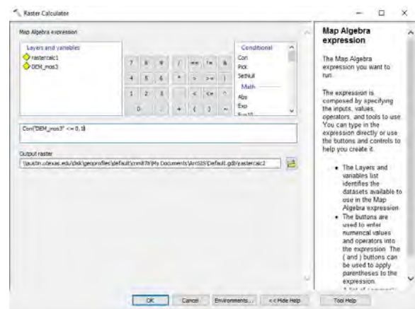
Figure 5: The Raster Calculator was used to create binary rasters for each sealevel, producing a raster that only had values where the land was beneath 0 ft.
