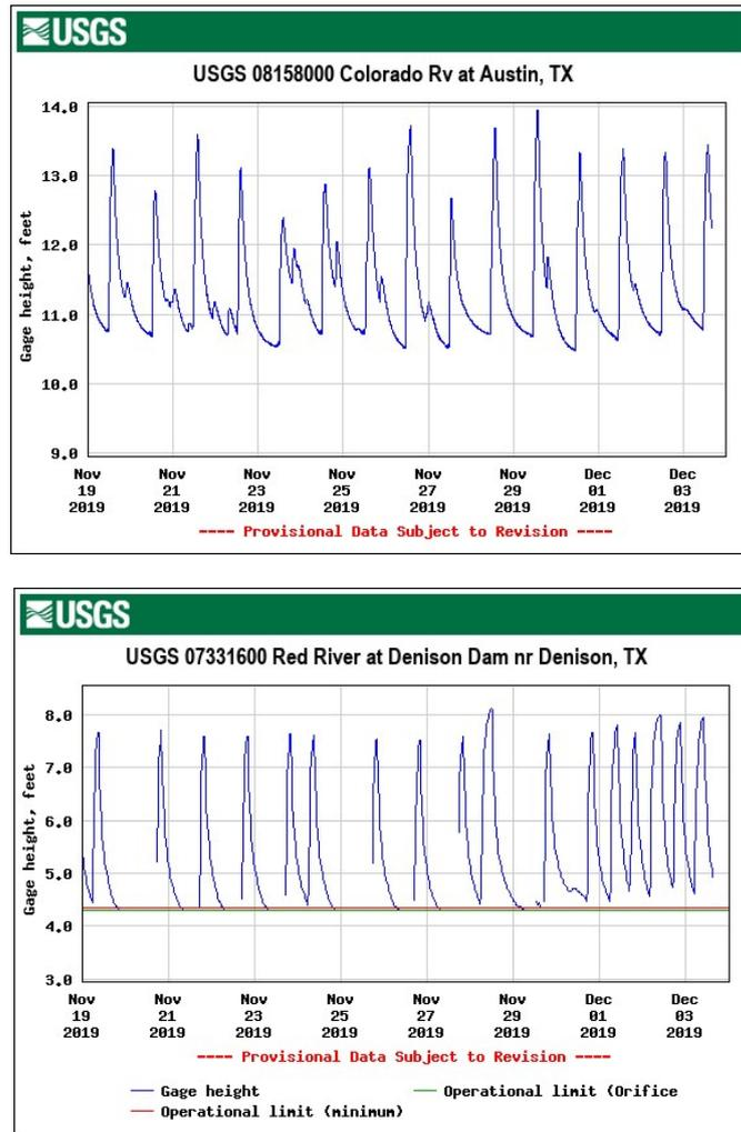
Figure 1.2: Hydropeaking in the Colorado and Red Rivers as a result of upstream dam operations. Graphs courtesy of USGS.
