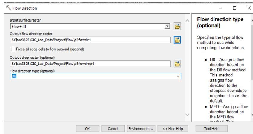
Figure 11. Turning the smooth elevation file into an flow direction profile.
