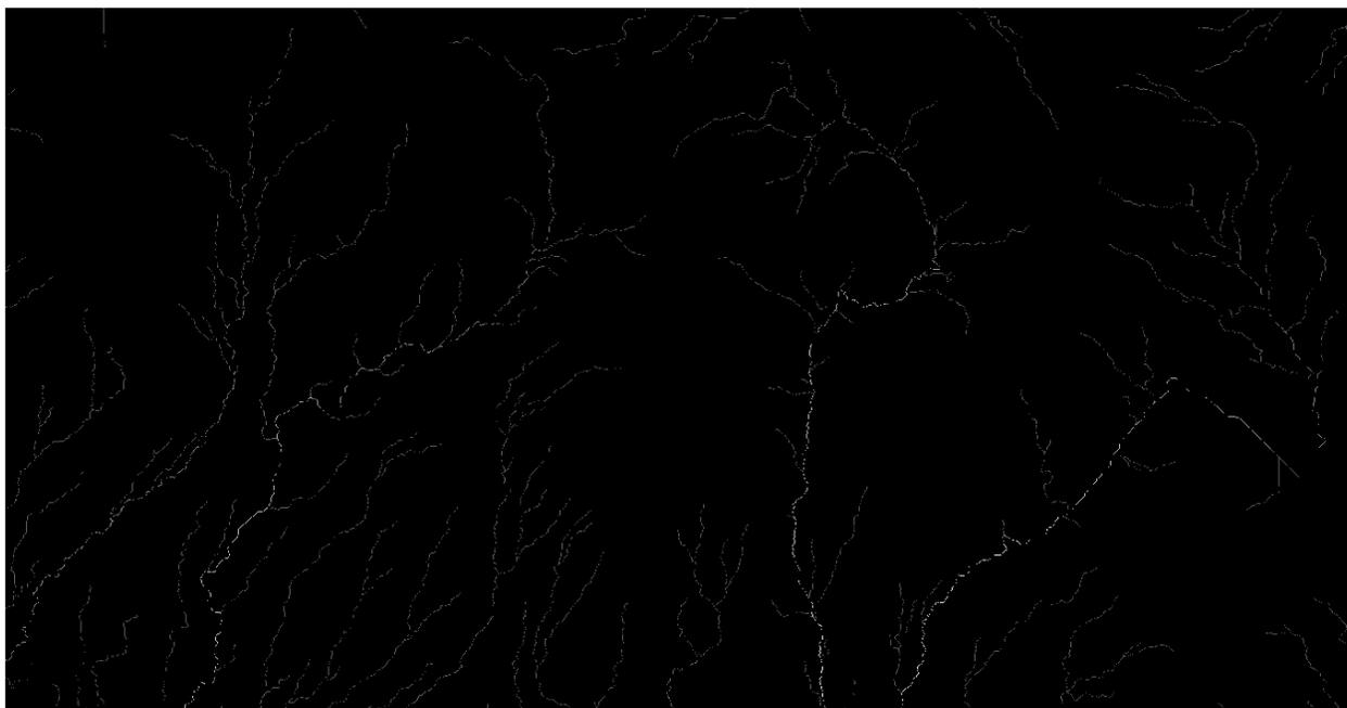
*Figure 13. Flow Accumulation. A ranking of how powerful flow is based on how many streams discharge into a single stream. The brighter the line or area, the greater the flow. The symbolization has been enhanced for visual ease.*
