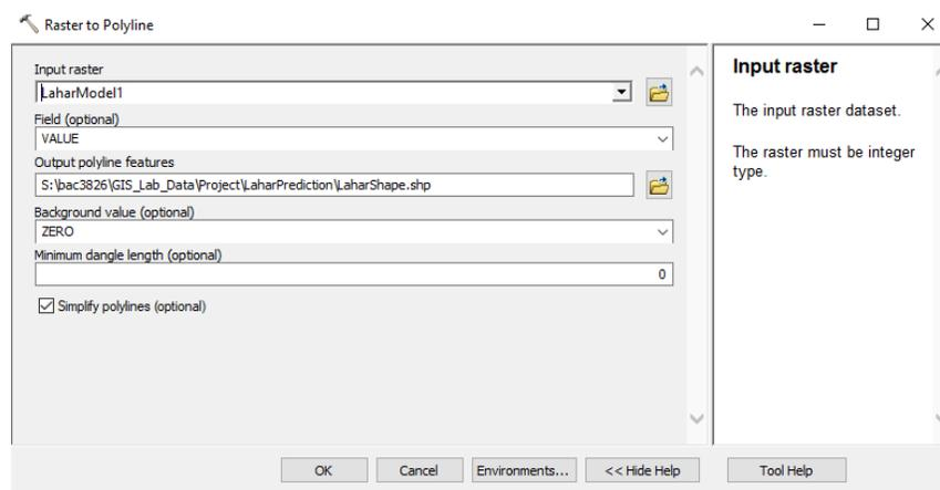
Figure 18. Converting Lahar Raster File into a Line Shapefile. The same is done for the rivers raster.
