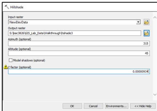
Figure 8. Conversion of Elevation Data into a Hillshade to Demonstrate Data on a Map.
