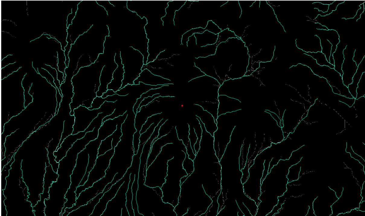
Figure 14. River shapefile, previously loaded in, overlain on Flow Accumulation raster to demonstrate accuracy of flow generation.
