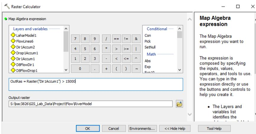
Figure 15. Raster calculator to form new binary rasters. Values over 15000 will generate a flow path of all rivers. Values over 60000 will represent a stronger accumulation of flow which are more likely to serve as Lahar flow pathways
