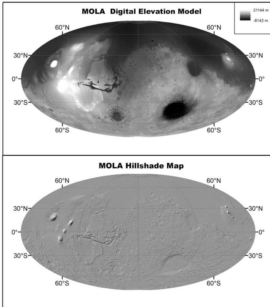
Figure 1. (Top) DEM from MOLA shotpoints. (Bottom) Hillshade map created from MOLA DEM. Both maps have a Mollweide Auxiliary Sphere projection with a GCS Mars 2000 coordinate system.
