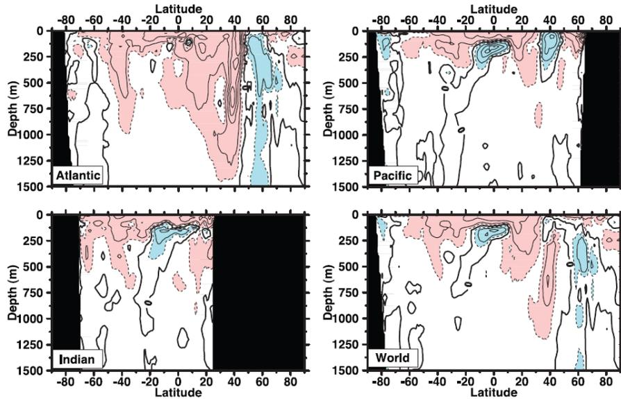
**Figure 3:** Longitudinally-averaged temperature anomalies as a rate of change per decade. Red areas indicate warming greater than  $0.25^{\circ}\text{C}$  per decade, while the blue areas indicate cooling greater than  $0.25^{\circ}\text{C}$  per decade. Figure taken from [1].
