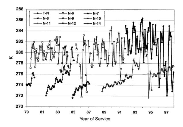
Figure 27: Monthly average MSU Channel 2 Hot Calibration Target temperature as measured by the two platinum resistance thermocouples (PRTs) monitoring it for each of the individual MSU's during the satellite era. This represents the temperature of the instrument itself. Variations in this temperature can be used to estimate the magnitude of IBE impacts on MSU2 trends. From Christy et al., 2000.
