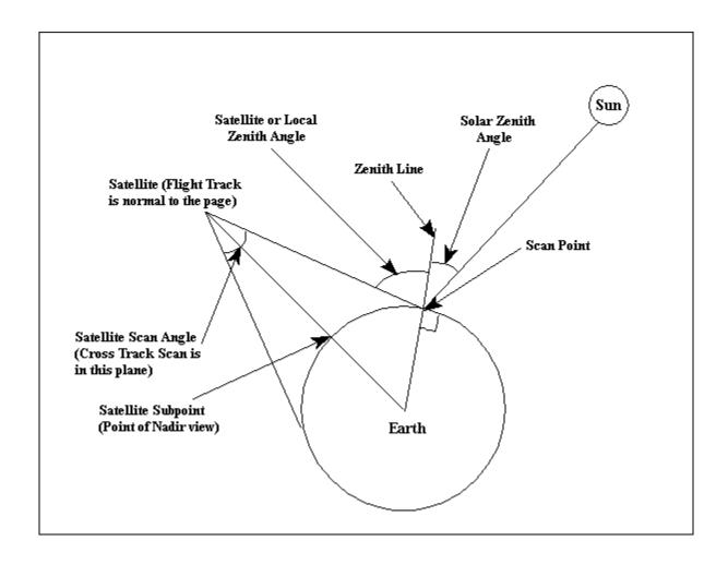
**Figure 5:** POES Satellite Flight Path and Scan Geometry in the ecliptic (Sun/Earth) plane. The north pole is normal to the page.
