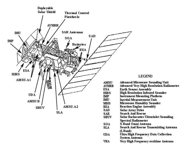
**Figure 6:** The TIROS-ATN Spacecraft and its components. The A1, A2, and B Advanced Microwave Sounding Units are the packages used for troposphere and stratosphere temperature studies.
