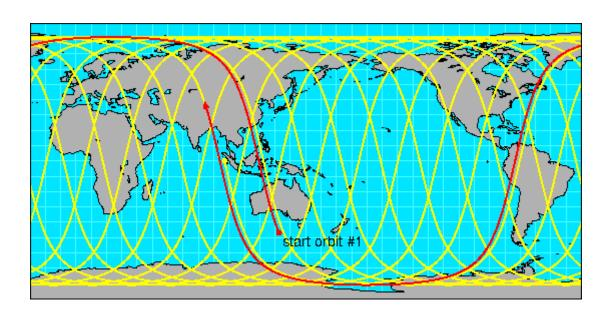
**Figure 4:** POES Satellite Flight Path with respect to the earth's surface.
