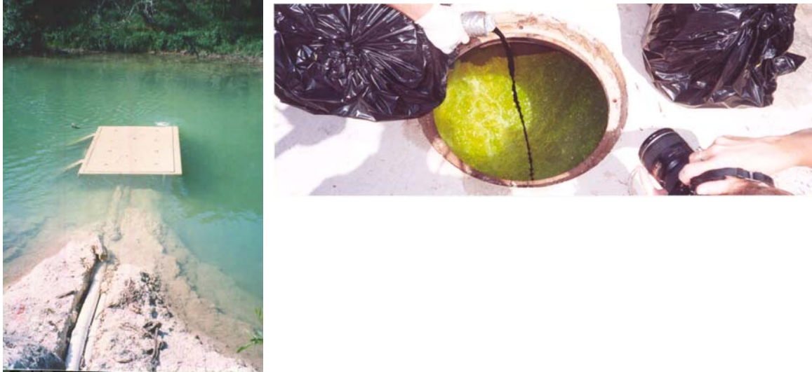
Figure 2. Concrete vault and valve system above Antioch Cave within Onion Creek (left). Sodium fluorescein dye being poured into the top of the vault (right).
