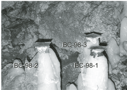
Figure 2. Experiment with glass plates at stalagmite sites BC-98-1, 2, and 3 in the Upper Passage of Harrison's Cave, Barbados, West Indies. Individual glass plates measure 10 cm × 10 cm.
