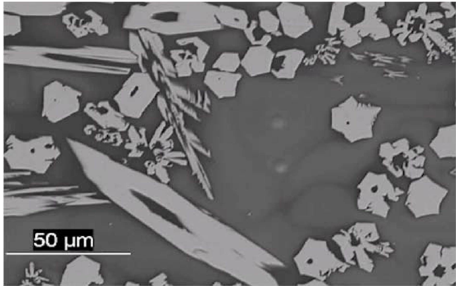
Fig. 3. Enlarged image of the central area in Fig. 1. The Gd-silicate apatite crystals are elongated, acicular, prismatic or dendritic; cross-sections are often hexagonal. The average size is tens of \mu\text{m} , but some crystals are up to 200 \mu\text{m} in length.
